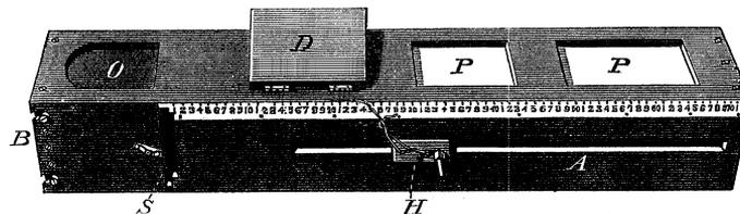
To hold the screen a box was constructed, as shown in fig. 2. It was made as light as possible, panels of card (as at P, P) being used instead of wood when practicable. The glow lamp to be employed was fixed in a holder inside the box; this could move along the slot A, and be fixed by a thumbscrew, H, in any desired position. (It may here be remarked that the plane of the filament was at right angles to the axis of the tube.)
