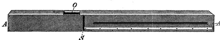
similar slot for the lamp as in the other instrument. The end A was, however, open, and during the eclipse it was placed at such an angle that the axis of the tube pointed to the centre of the Moon. The aperture, O, for making the observations was in this case also covered with a black velvet cloth, under which the head of the observer was placed.
